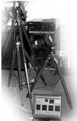
All that's listed became a single stone including the floor<sup>15</sup> except the camera. This is the ideal vibration-free camera support setup. If I remember right, Ansel Adams was carrying a big solid concrete block to make the support stable.<sup>16</sup> Precision machine tools always sit on top of the big solid epoxy granite bed.
